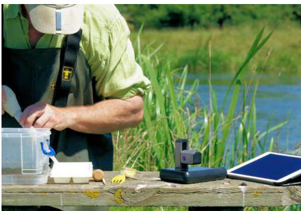
Portable microscopes can capture and share images and videos of parasites and other fish pathology instantly
