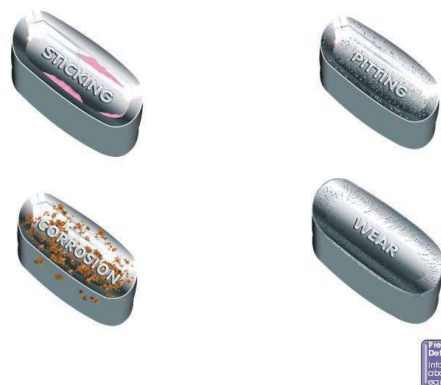
Figure 1 - Issues you might encounter (Sticking, Pitting, Corrosion, Wear)
