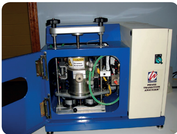
Photo of table-top lab equipment. Phase transition analyser.
